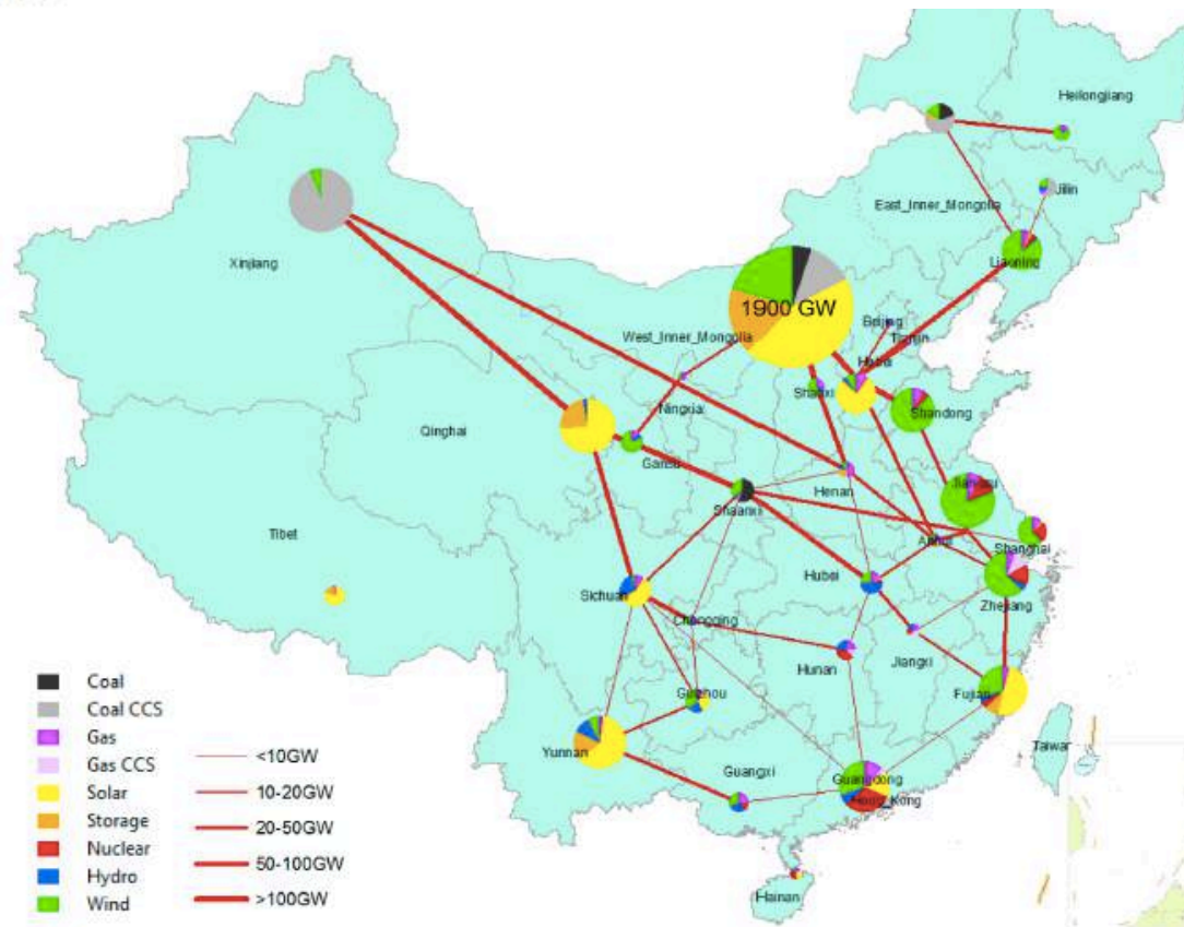
Figure 4. Generation, transmission, and storage capacity needed to achieve an 80% carbon reduction in 2050. All represented lines are new transmission expansion. Inner Mongolia emerges as a major center of clean energy generation thanks to the combination of its location (a few hundred kilometers from major demand centers) and high-quality renewable energy resources.
